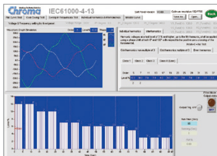
Voltage Harmonic & Interharmonic Test
