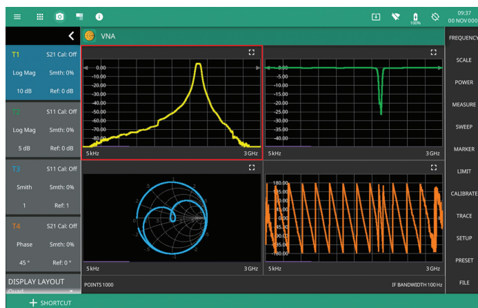
Quad Display Highlighting Essential Characteristics of a Bandpass Filter
