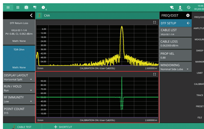
Split Screen Showing DTF and TDR Measurements
